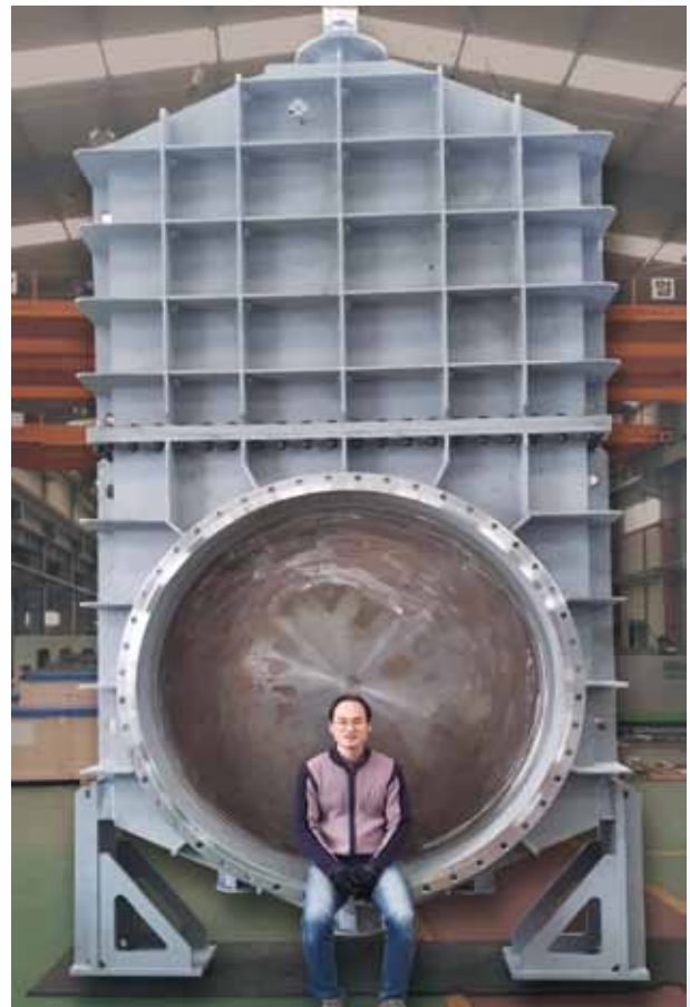
WELDING TYPE GATE 2000A to POSCO #2 BFG GAS PJT
