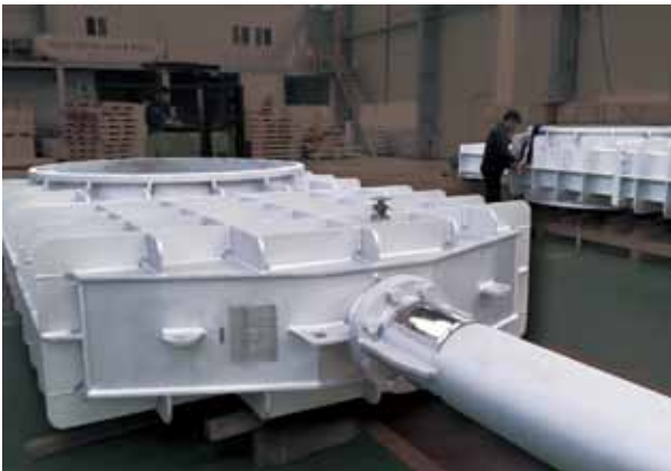
WELDING TYPE GATE 2000A to POSCO #2 BFG GAS PJT
