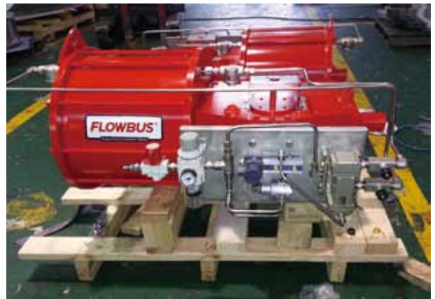
POSCO POHANG CCPP - SHUT/OFF VALVE (PNEUMATIC ACT)
